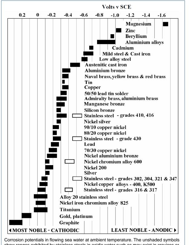
show ranges exhibited by stainless steels in acidic water such as may exist in crevices or in stagnant or low velocity or poorly aerated water. The more Noble materials at the left side tend to be cathodic and hence protected; those at the right are less Noble and tend to be anodic and hence corroded in a galvanic couple.
