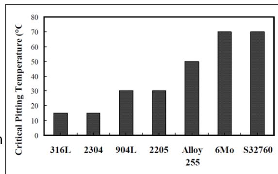
A commonly used test is that in ASTM G48, which measures resistance to a solution of 6% ferric chloride, at a temperature appropriate for the alloy, shown in the graph above. If an artificial crevice is added to the sample the test measures crevice corrosion resistance rather than pitting resistance. The temperature which is just high enough to cause failure of this test is termed the Critical Pitting Temperature (CPT) or the Critical Crevice Temperature (CCT).
