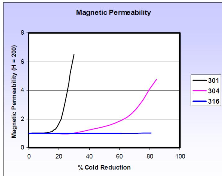
These comparisons are shown in the graph above. Note that different heats of steels of the same grade may exhibit different magnetic responses because of minor differences in the amounts of each element.
